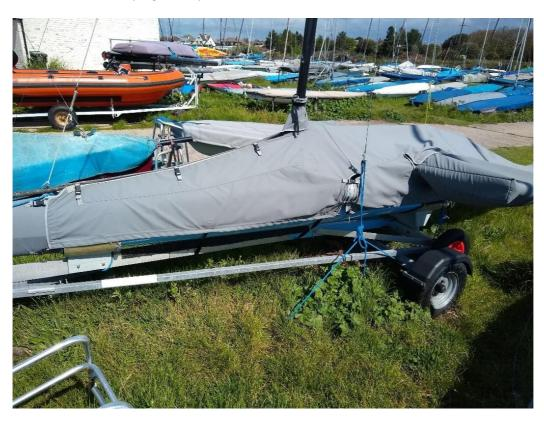
For dinghies with unstayed masts and flat covers (eg Lasers and Toppers), which do seem to be least concerned about tying down, ties should be about third of the way from the bow to the trolley wheels and ideally a bow tie down as well, as demonstrated by the Aero in the photo below.
