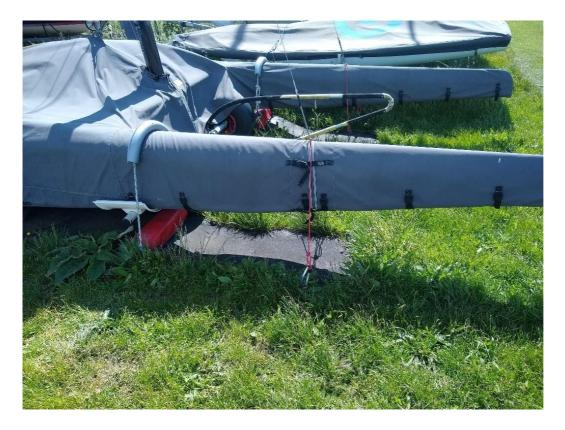
In winter, boats are best taken away from the club and stored under cover. If left at the club unchecked, it is **essential that the mast is taken down and laid in a safe place.** The boat cover should be securely tied on with support so water drains off. Another option is to turn the boat upside down, tied down and raised off the ground. Take a look around the compound to find examples of good practice to protect your boat and your fellow members' boats around you.
