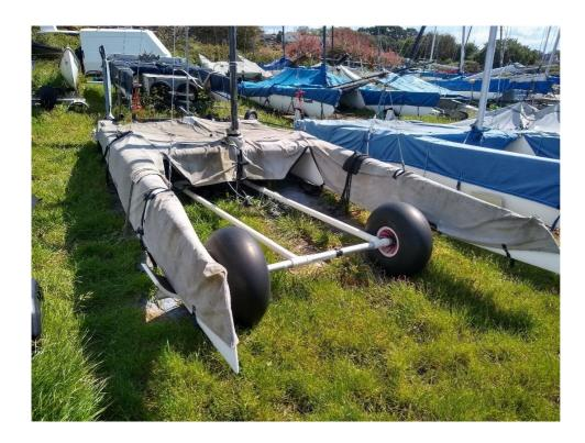
In addition, due to the catamaran's higher windage, they do need a minimum of two anchorage points i.e. one at the bow and one at the transom. A mid point tie down is not sufficient. Note also the padding to protect the hull from damage by the tie down cables.
