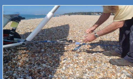
Step 6 With both lines extended, bring trolley buggy to meet your boat trolley
